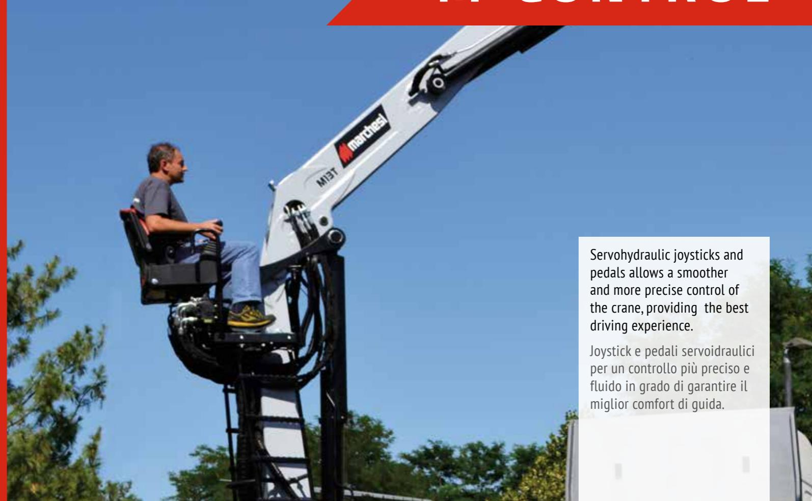
Servohydraulic joysticks and pedals allows a smoother and more precise control of the crane, providing the best driving experience.
