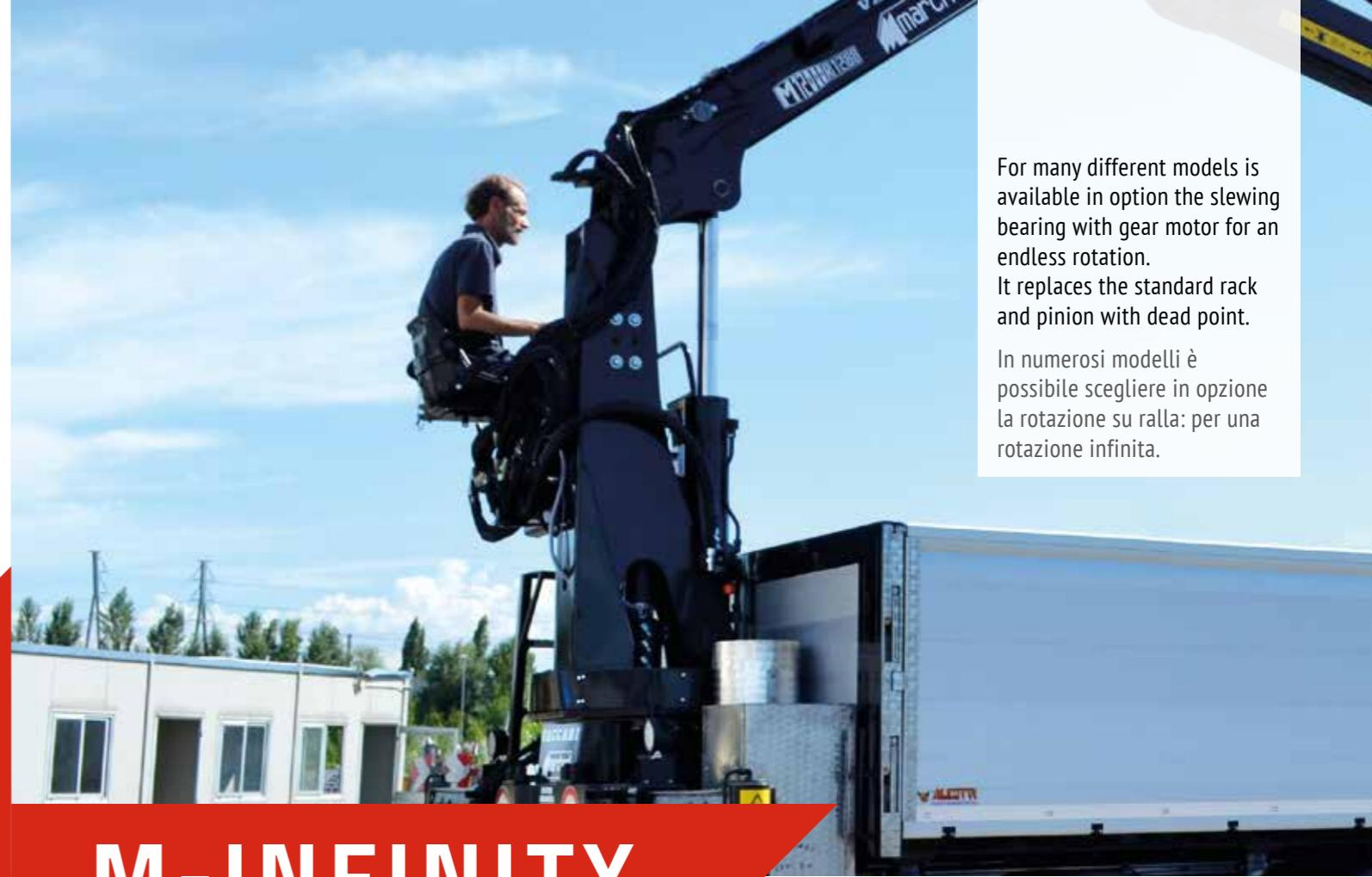
For many different models is available in option the slewing bearing with gear motor for an endless rotation.
