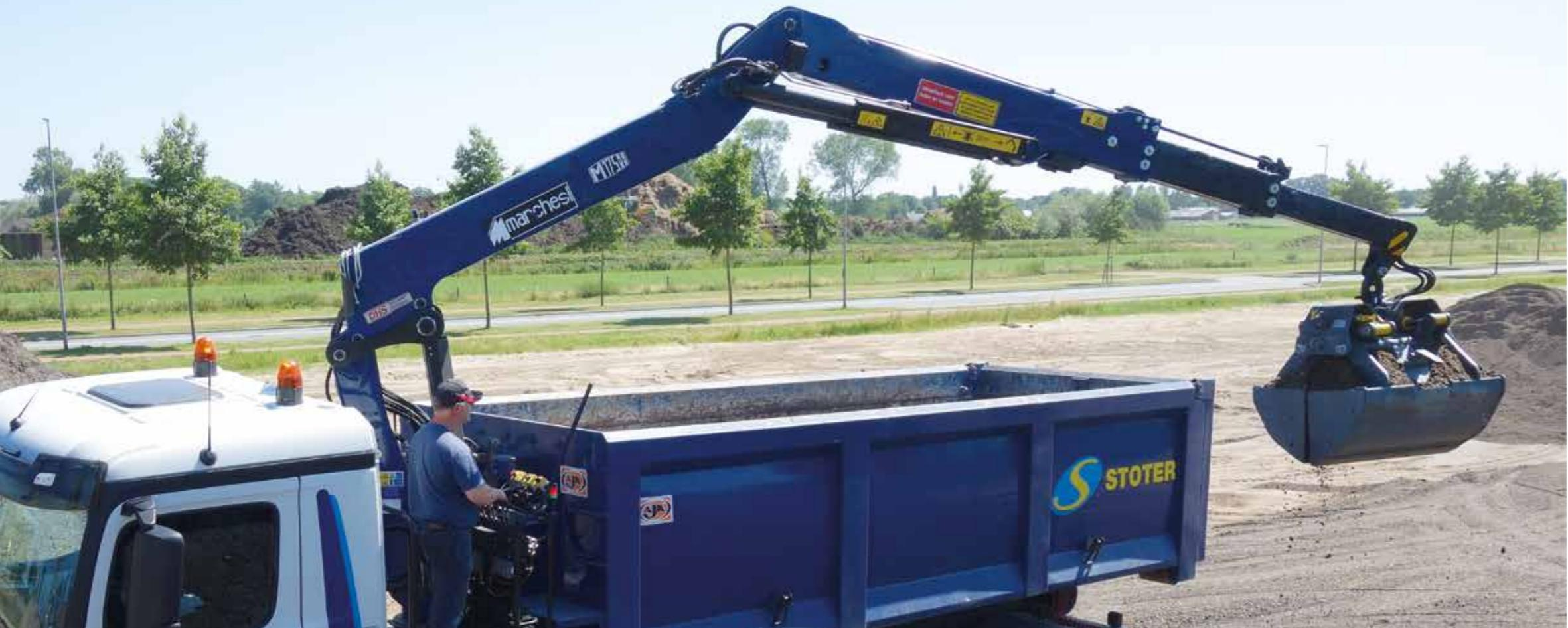
Cranes in Z-type with a new geometric design of the booms that allows a great outreach (until 9.20 meters) without going below the truck frame. The best solution for the new trucks and for installations on demountable containers.
