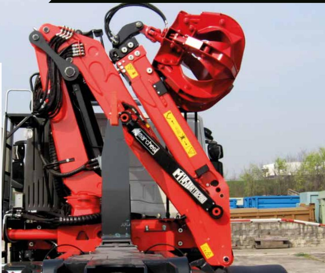
Our design grants the possibility to fold the crane together with its attachment even with a large polyp grapple while remaining in the width of 2.55m.
