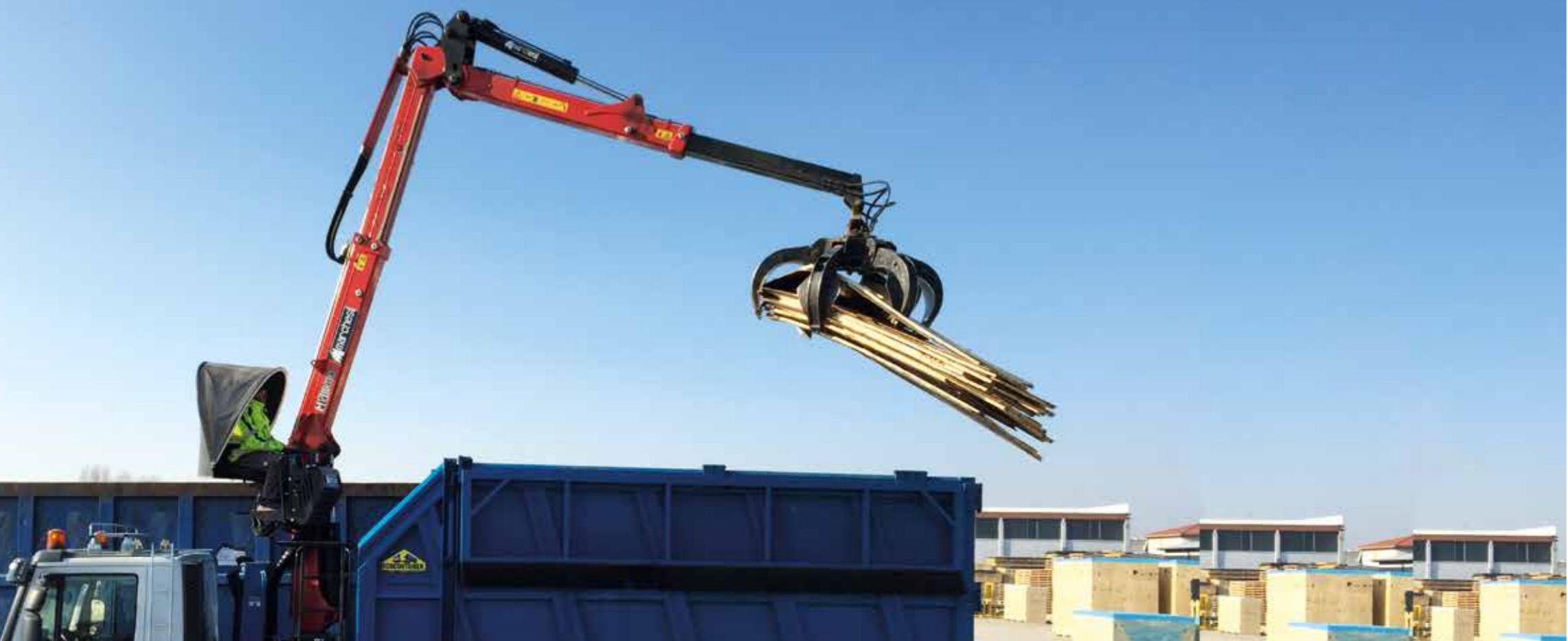
These cranes in L-Type are equipped with M-Extra, the telescopic first boom that allows a great flexibility during work as a greater loading capacity in height.
