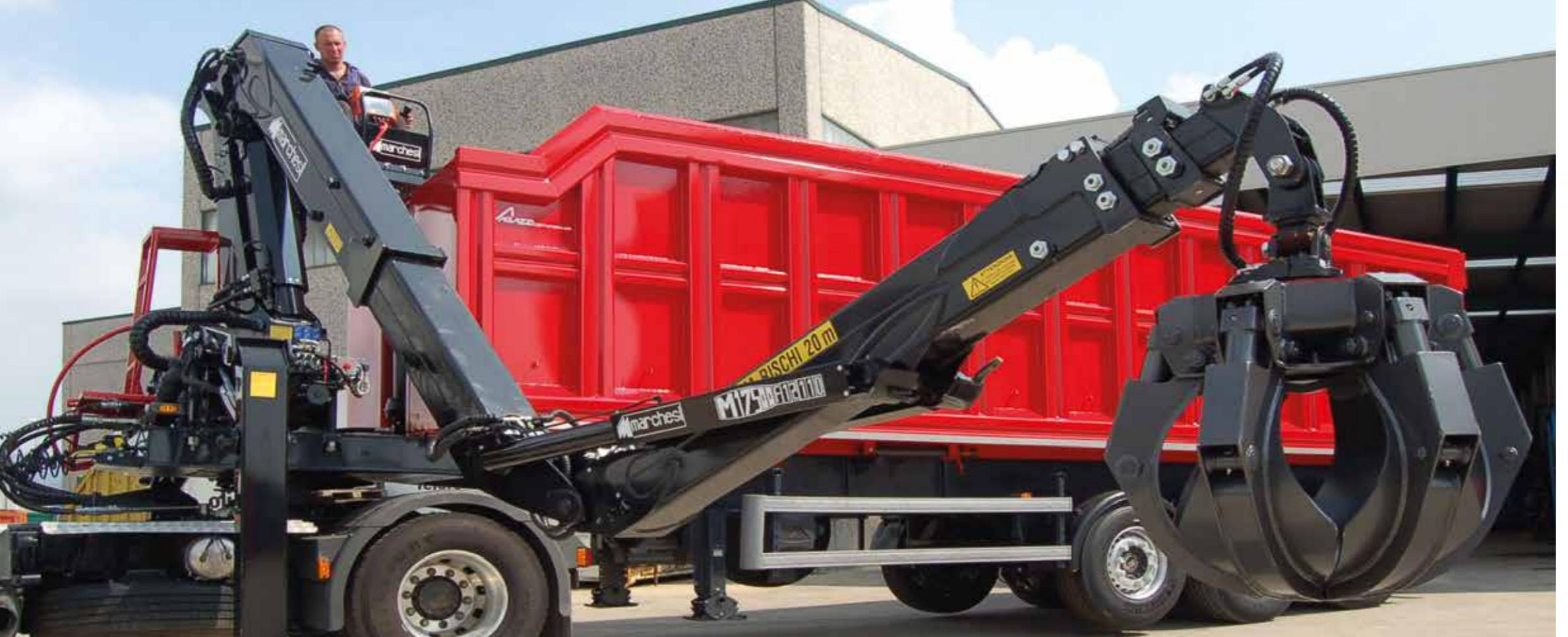
Cranes in Z-type with the M-EXTRA (telescopic first boom) have a great versatility and an excellent outreach until 10.5 meters. All the cranes in this class don't go below the truck frame when are in transport position; a feature especially appreciated on new trucks.
