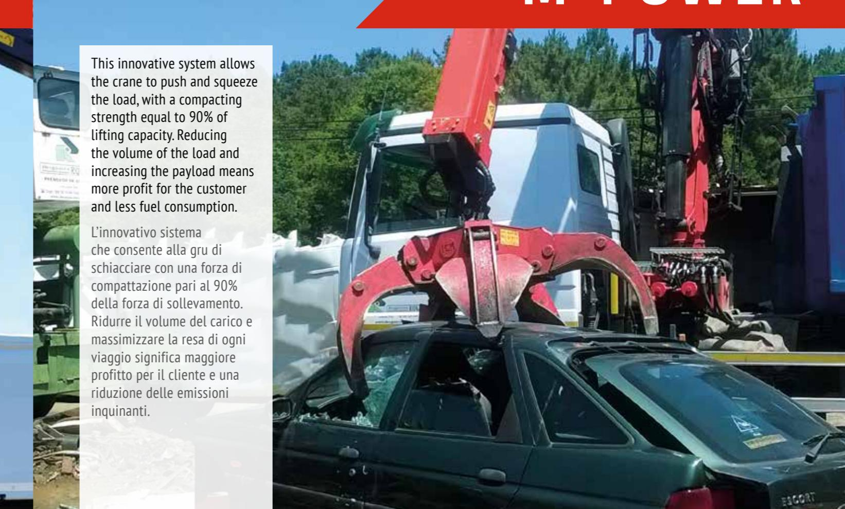
This innovative system allows the crane to push and squeeze the load, with a compacting strength equal to 90% of lifting capacity. Reducing the volume of the load and increasing the payload means more profit for the customer and less fuel consumption.
